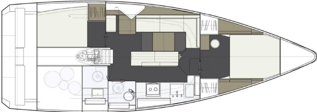
VERSION 111 – STANDARD 2 Cabins, 1 aft Head, 1 Toilet
